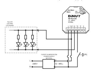
· Pushbutton connected to 230V:
