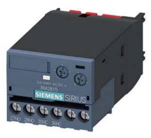
Solid-state time-delayed auxiliary switch OFF delay without control signal Relay 1 NC + 1 NO 24...240 V AC/DC Time range 0.05...100 s Can be snapped on at the front For 3RT2 S00-S3 contactors and 3RH2 S00 contactor relays Screw terminal Varistor for attenuation of the contactor coil integrated
